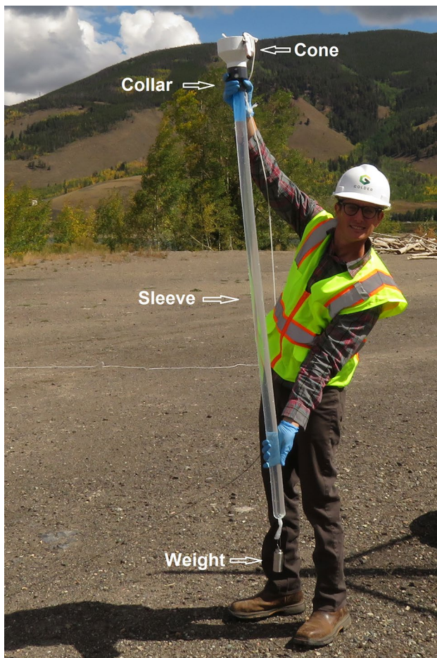
Fig. 2 A full, 1.5-m-long HydraSleeve after drone sampling
